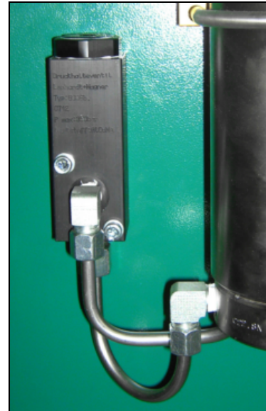
Pressure Maintaining Valve
