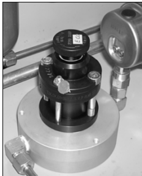
Endpressure Safety Valve
