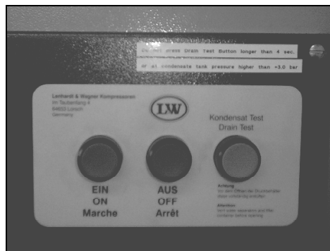
Start / Stop Keys & Condensate Drain Test Button (Standard Control System)
